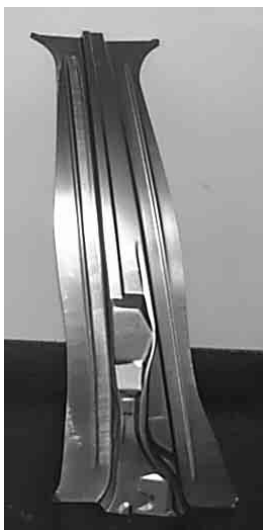
Photo 3 Applied example for center pillar reinforcement of TS980 MPa steel (lor YR type) (Formed by the experimental stamping tools in JFE Steel)
